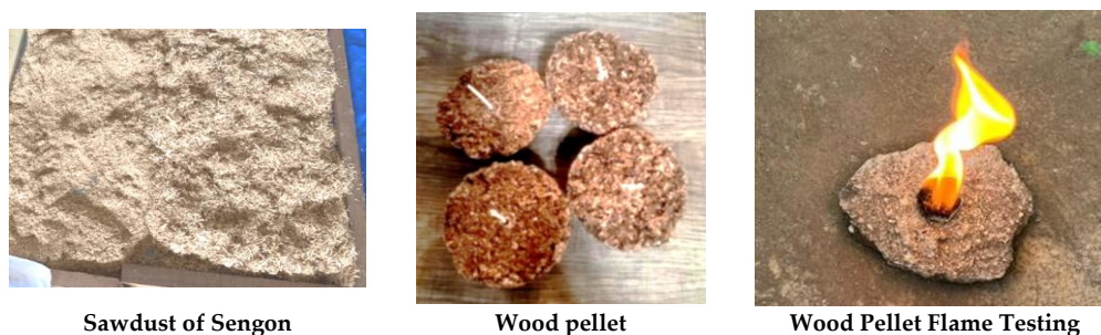
Figure 3. Wood Pellet Making and Wood Pellet Flame Testing
