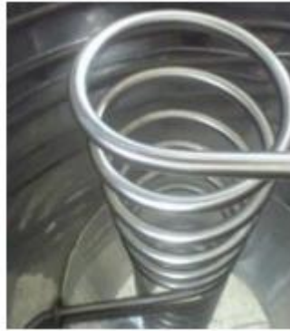
Figure 4. fluid pipes in condensers
